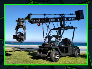
Custom built electric camera platform, silent with zero emissions.
