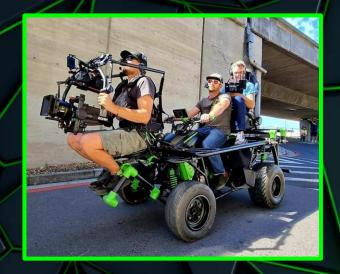
400CC Quad Bike with custom chassis, offering various grip friendly rigging points. Can be used for Hand-Held, Steadicam and Hard Mount setups. With on and off-road capabilities, the Cricket is a compact and versatile machine. Offering, front and back, height adjustable, rotating, GFM spring rig, with hard mount, stabilised head capability.
