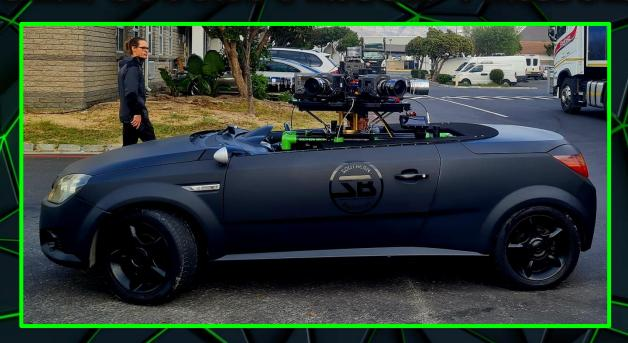
Our Tigra Plate vehicle offers both stabilised and hard-mount rigging options with lens heights from 1100mm to 2800mm. She has an on-board power supply (12v & 240v) for ancillary equipment as well as ample boot space for additional batteries. Super smooth suspension and wider profile tyres allow for speeds up to 140 km/h on various prepared surfaces. The Tigra is fully licenced and insured to operate on national roads.
