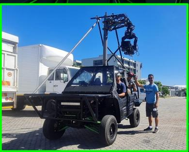
Our 6Ft Pole Mount System from Grips Factory Munich sets the bar when shooting with a Hard-Mount Setup. Working in conjunction with our Maxi Vibration Isolator it has a payload compacity of up to 100KG.
