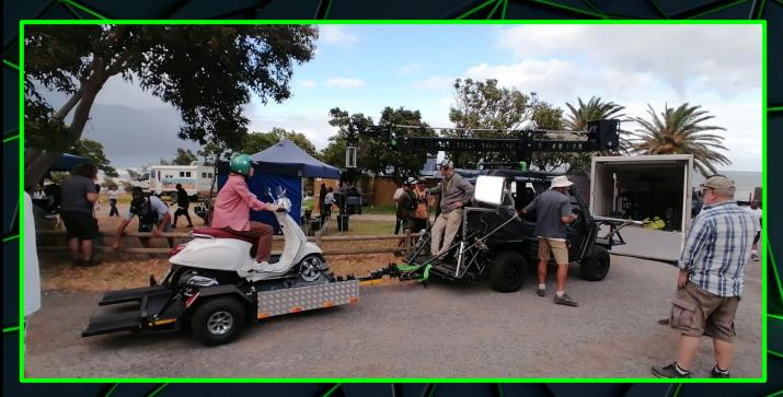
Our Low-Loader Bike Trailer, is perfect for process work with both motorbikes and bicycles. With a load compacity of up to 500Kg and a ground clearance of just 8 inches. The trailer can be supplied with two side platforms to increase the working area if required. Various lockdown points are available, and it is fully licenced and insured to operate on the national roads.
