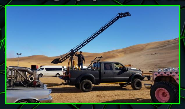
A strong, reliable, double cab, 4X4, tracking and support vehicle. With a custom aftermarket suspension system, giving the F250 superior ground clearance and traction capabilities.
